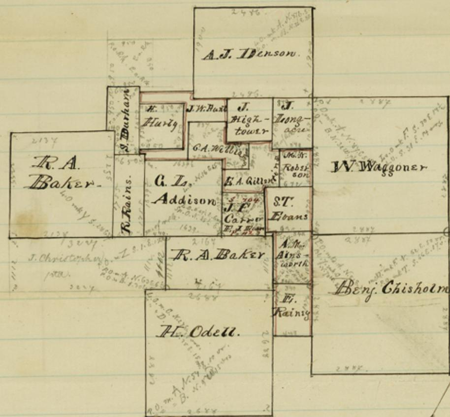
I S. S. Evans County Surveyor of Breath County do hereby certify, that from actual measurement upon the ground, I find a space of 840 acres between the R. A. Baker and H. Odell surveys, and the Benj. Chisholm survey, and that the above map is a true representation of surveys made by me, for a description of which reference is made to accompanying field notes.
